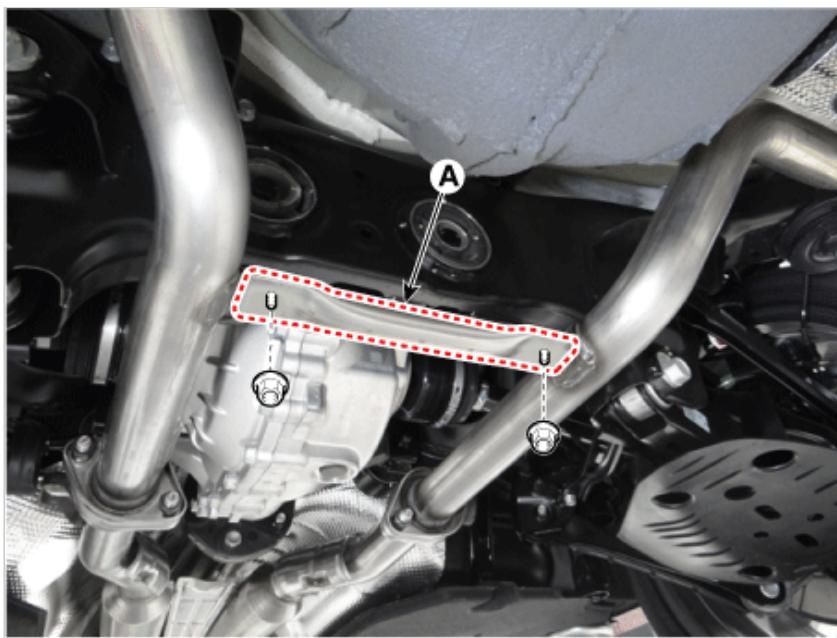
2. Detach the hanger (A) from the RH rear muffler.
