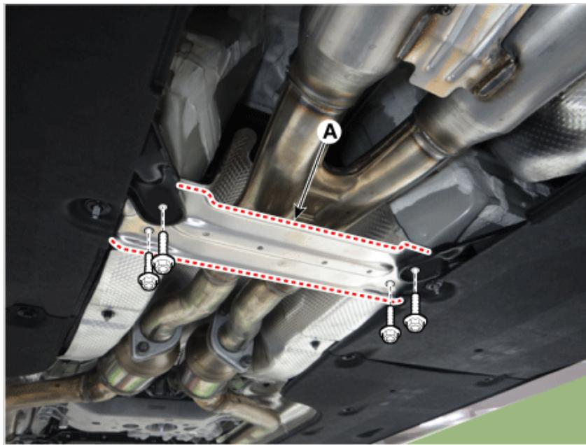
2. Remove the rear muffler bracket (A).
