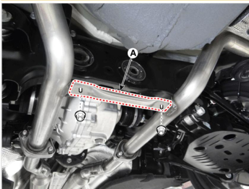
3. Remove the front muffler bracket (A).
