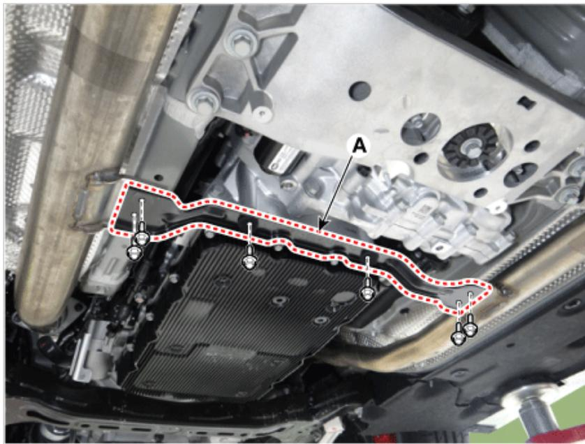
4. Remove the RH front muffler (A).
