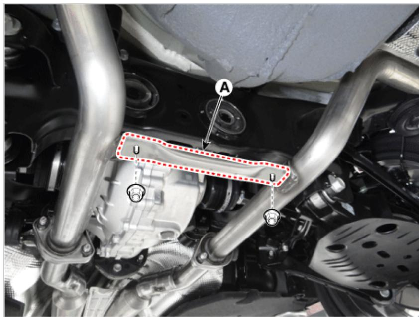
2. Detach the hanger (A) from the LH rear muffler.
