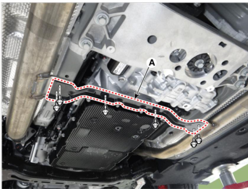
4. Remove the LH front muffler (A).
