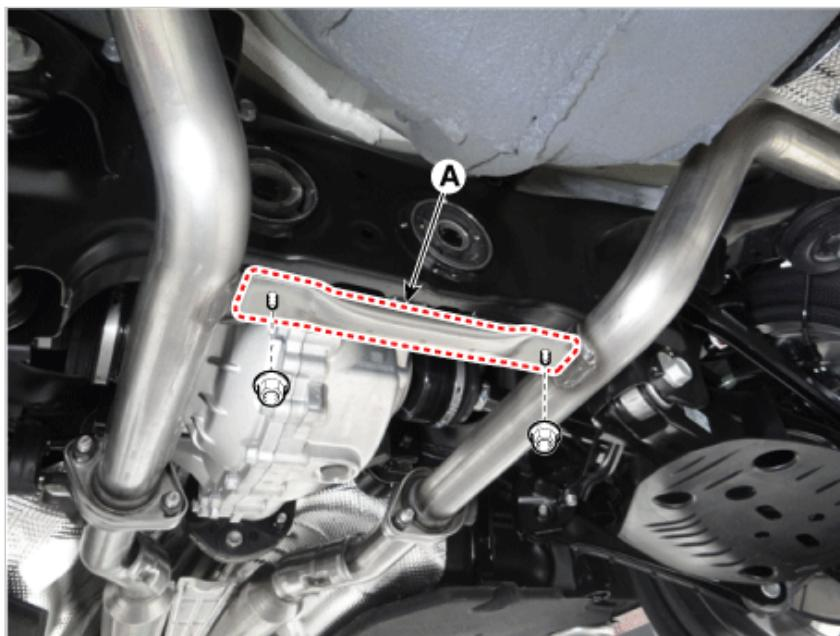
3. Remove the front muffler bracket (A).
